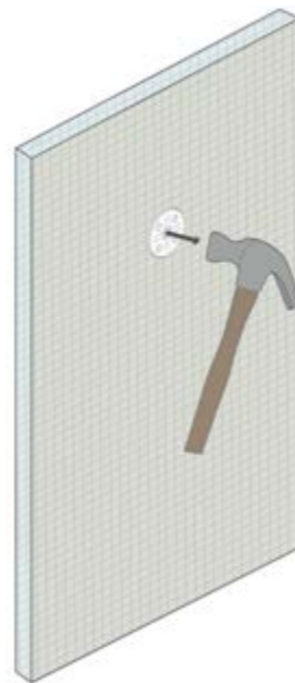
Fig.2 Hammer home all fixing pins until the Orbry™ Spanker Dowels are all securely fixed.
