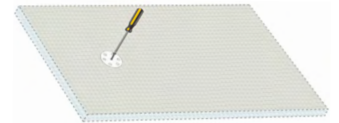
Fig. 19 For timber floors, mechanically fix the Orbry Boards at 300mm centres using Orbry Stainless Steel Screws and Orbry Tile Backer Board Washers.
